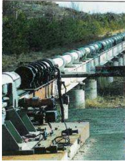
Figure 2: Aerobut testing equipment
