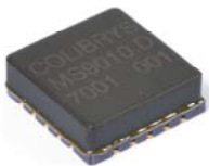
Figure 1. Colibrys extra small LCC20 packaging (8.9mm x 8.9mm)
